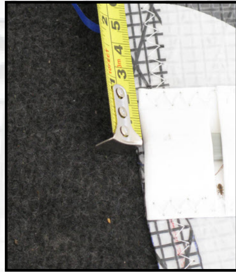
Each batten spacing should be measured to the centre of the batten pocket
