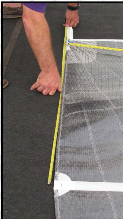
Measure between all battens and also measure the the bottom spacing to the tip of the clew, not the cringle
